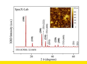
XRD, AFM of ITO/SnO2/ FAPbBr3/PTAA/ITO top cell. Perovskite deposition by Spin on SnO2 by blade
