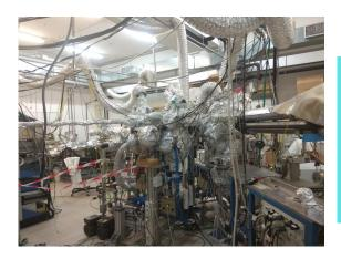
Integrated UHV MBE1-UPS-IPES-AES System for Perovskites/HTL/ETL Epitaxial Growth and Structural/Electronic Investigations.
